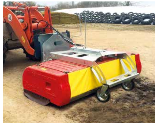
The big collecting box picks up large amounts of dirt.
